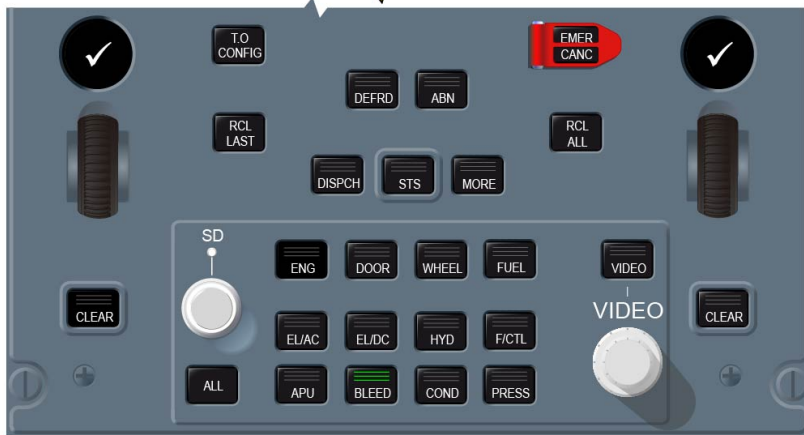
ECAM CONTROL PANEL
