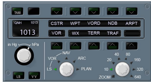
CAPT EFIS CONTROL PANEL
