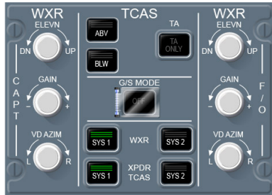
AESS CONTROL PANELS
