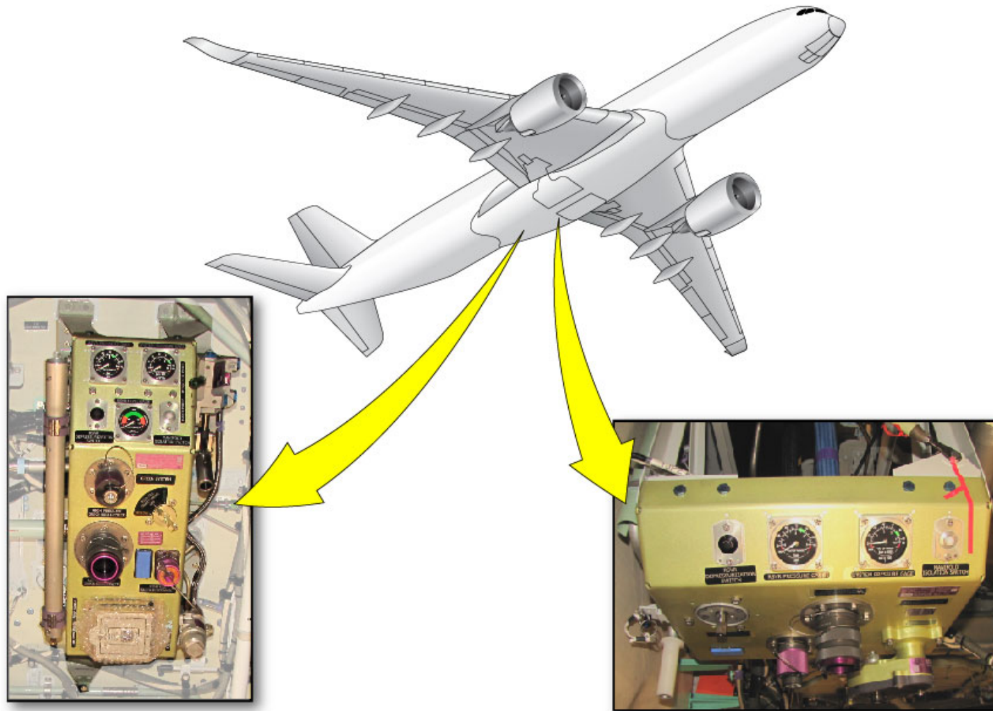
GREEN GROUND SERVICE PANEL
