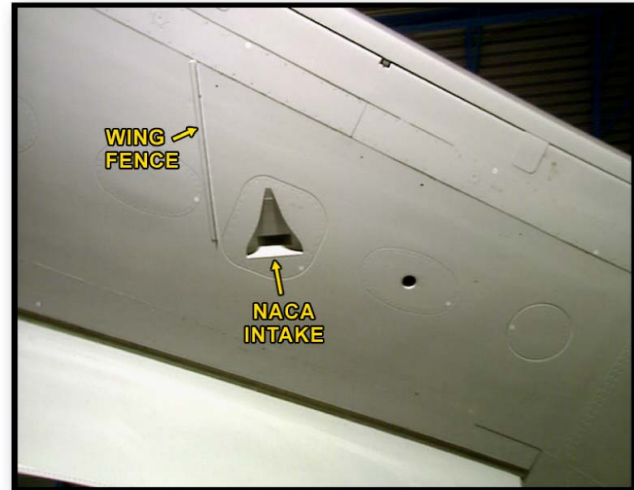
Wing fence and Naca air intake
