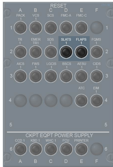
LEFT RESET SWITCH PANEL
