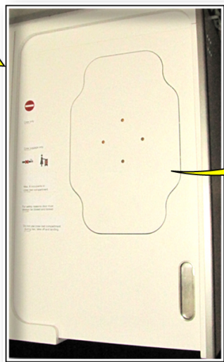
CABIN CREW REST COMPARTMENT SLIDE DOOR OUTSIDE VIEW
