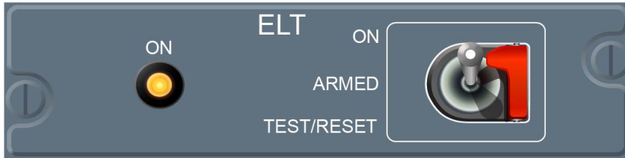
ELT REMOTE CONTROL PANEL
