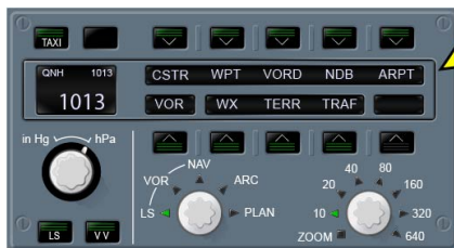
CAPT EFIS CONTROL PANEL
