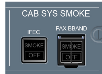
CABIN SYS SMOKE PANEL
