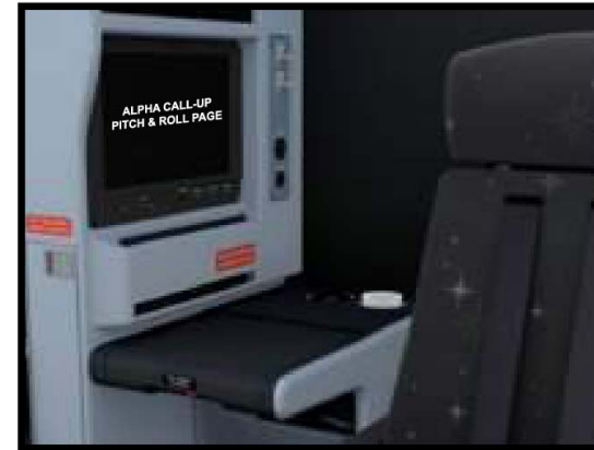
AIRCRAFT QUICK LEVELING FROM THE COCKPIT (WITH THE ONBOARD MAINTENANCE TERMINAL)
