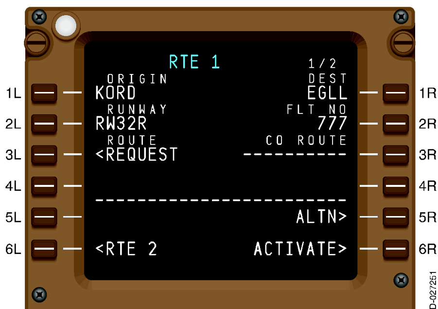
RTE 1 – Origin, Destination, Runway, Flight Number Entered Figure 4-18
