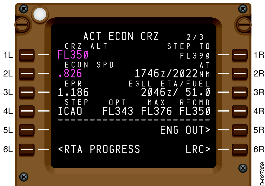
ACT ECON CRZ Page – Engine Failure. Figure 9-1
