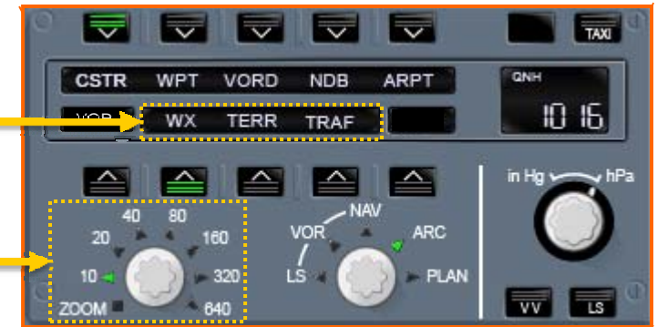
EFIS Control Panel
